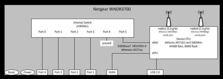
Physical port numbering does not equal logical port numbering
